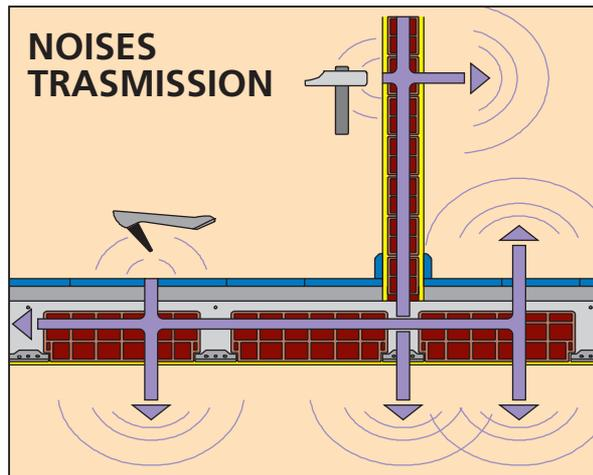
**Airborne Noises:** they are transmitted through the air that is moved directly by the vibrating source (vocal cords, loudspeakers, household appliances, etc.). Usually they affect the environments next to the one in which the source of the noise is localized. In this case the energy is relatively modest.
