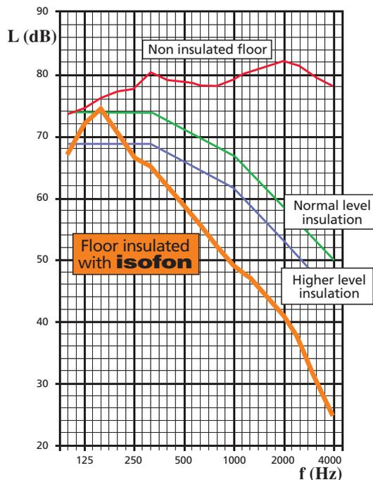
**isofon** is a product made up essentially of rubber bound with latex and layed on a bituminized paper support; it is design to obtain high acoustic dampings and very good 'floating floors'. Its characteristics are the following:
